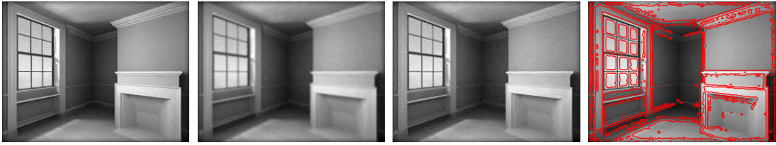
Figure 5. Images from left to right are: the original image, the observed blurry and noisy image \mathbf{f} , the reconstructed image using the PS algorithm, and the estimated jump set which is enclosed in the red curves.
