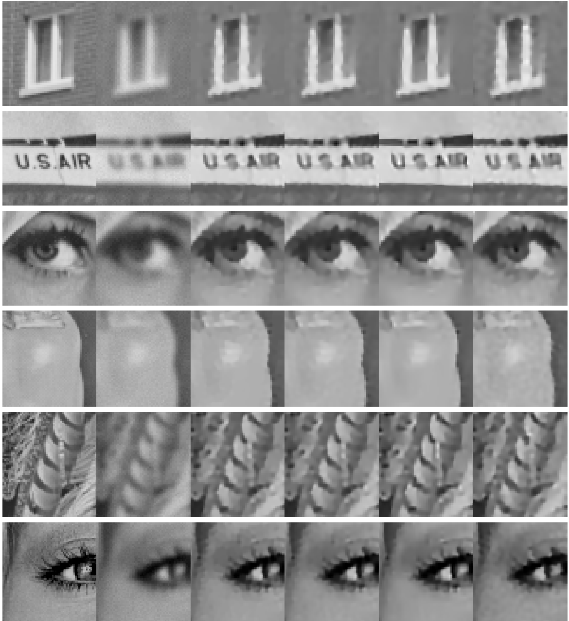
Figure 5: Zoom-in views of the processed results. From left to right: original images, noisy and blurred images, results of analysis based approach in (43), results of balanced approach (1), results of EPIHT-LS for (9), and results of SNC(ii).
